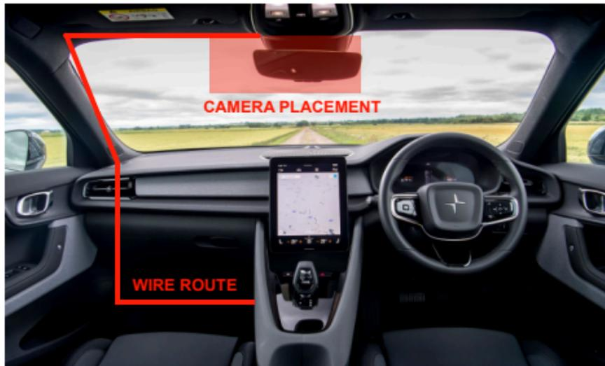
7. Ensure that the power cable is neatly tucked into the roof of the car, along the rubber tubing along the side of the door and under the lower part of the dashboard to the cigarette lighter socket. This will ensure that there are no loose wires in the vehicle from the dash camera to the power supply.
